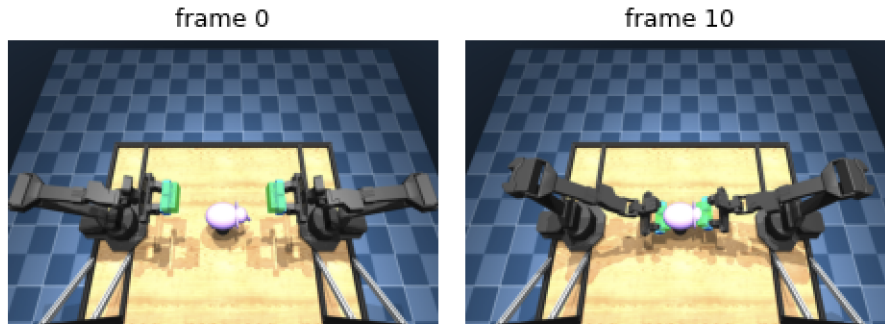
Figure 2: Top-camera frame strip for a toy_elephant episode. The scene contains two arms, a pedestal-mounted object, palm/fingertip touch sites, and wrist force-torque sites. The dynamics model does not receive camera pixels; it receives only the body-sensor vector.
